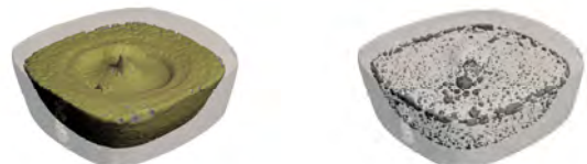
Figure 7: Visualization of composition of chocolate praline (left) and distribution of air bubbles (right)-
